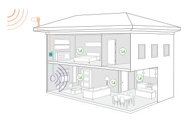
**Receives signal:** The outside antenna reaches out to access the existing strong outdoor cell signal and delivers it into the booster.
